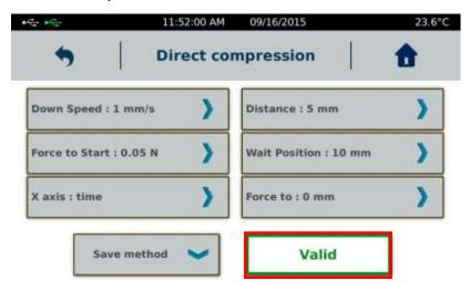
You arrive on this window (see below). Screw the holder onto the sensor and click on "Zero Force" to reset your force sensor to zero.
