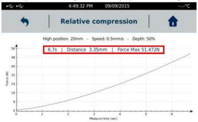
You could print the DATA results with a Dymo 450 TURBO (ticket format) or with an A4 printer compatible with HP PCL5 driver allowing the curve to be printed in this second case. You could also save your data by pressing the "SAVE" tab on screen. A file name will be asked to save it in the internal memory of the TX-700.
