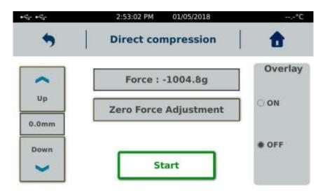
The accuracy of our force sensors is 0.05% of full scale. For example, a 50N sensor (5000g or 5Kg) allows a measurement with an accuracy of 2.5g [= (0.05x5000) / 100]. For a 500N sensor, the accuracy is 25g.
